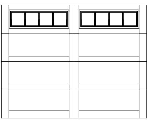
9' X 7' 6600 WESTFIELD DESIGN 4 SECTION/2 PANEL FRAMED STOCKBRIDGE TOP SECTION SHOWN CONSISTS OF (4) 20.8" SECTIONS
