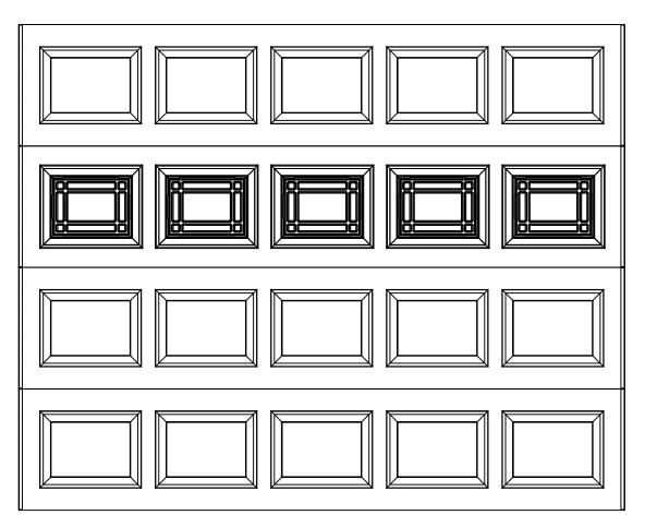
10 X 8 9605 CRP DESIGN 4 SECTION/5 PANEL PRAIRIE I INT3 SECTION SHOWN CONSISTS OF (4) 23.8" SECTIONS
