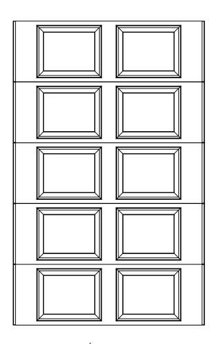
5 X 8 9100/9605 CRP DESIGN 5 SECTION/2 PANEL CONSISTS OF (5) 19.1" SECTIONS
