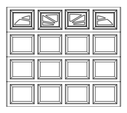
8 X 7 9100-9605 CRP DESIGN 4 SECTION/4 PANEL WILLIAMSBURG I TOP SECTION SHOWN CONSISTS OF (4) 20.8" SECTIONS
