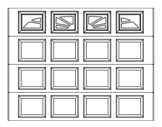
9 X 7 9100/9605 CRP DESIGN 4 SECTION/4 PANEL WILLIAMSBURG I TOP SECTION SHOWN CONSISTS OF (4) 20.8" SECTIONS
