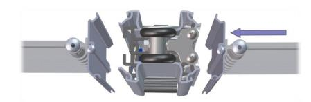
**Insert** the hook end of the connector into the slot on the post and rotate the curtain connector flat against the post.
