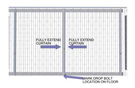
**Drill** the hole to accept the floor socket. Drill size:
