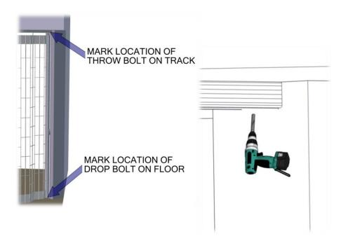
**Drill** the hole to accept the floor socket. Drill size:
