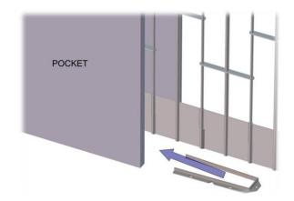
**Mark** the front mounting hole on the floor.
