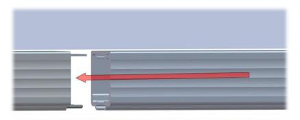
**Joint** must be tight with no gaps to ensure the trolleys do not catch and the door travels smoothly through the joint.
