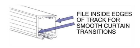
Track is pre-drilled for  $#10 \times 2''$  screws (provided).
