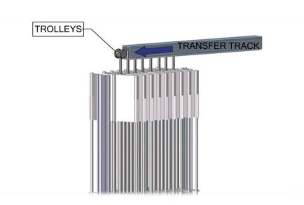
**Lift** the curtain and place the transfer track end-to-end with the installed track.
