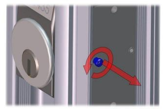
**Remove** the cylinder by unscrewing it counter-clockwise.
