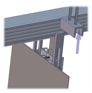
**Loosen** the hex bolts to adjust the height of the top stop.
