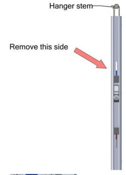
**The top lock rod** will always travel 1.5" from unlocked to locked, but the position is variable.
