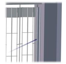
**Mark** the lock rod locations on the track and floor.
