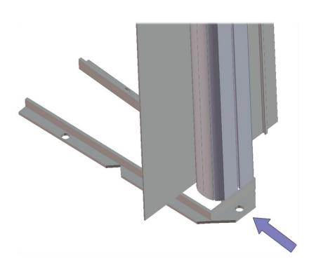
**Bend** the V-stop as required to fit the shape of the pocket
