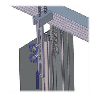
**Raise** the top stop so that it catches to ceiling stop. Leave as little clearance as possible between the top stop and the ceiling.
