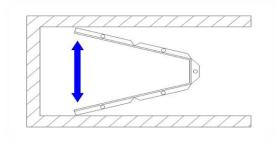
**Detach** trailing post from curtain (reverse directions in Step 5), and raise the bottom stop enough to pass over the V-stop.
