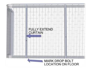
**Drill** the hole to accept the floor socket. Drill size:
