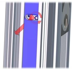
**Remove** the cylinder by unscrewing it counter-clockwise.
