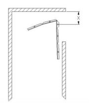
Drill a 1/4" hole, 1 1/4" deep where marked in the pocket. Replace V-stop and fasten using nail-in anchor provided.
