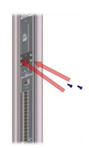
**Replace** the cover plate and retaining screw.
