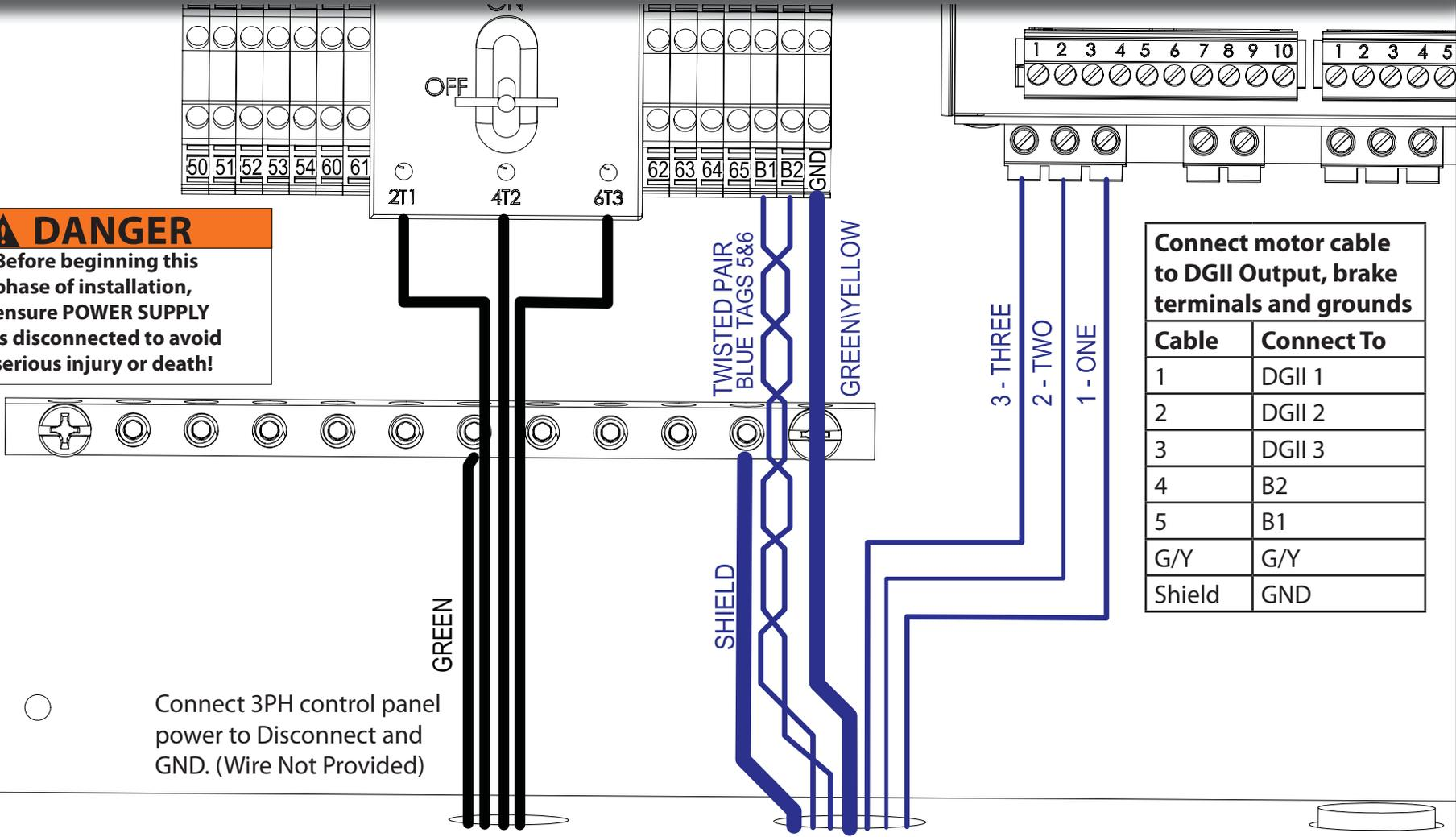
Connect motor cable to DGII Output, brake terminals and grounds
