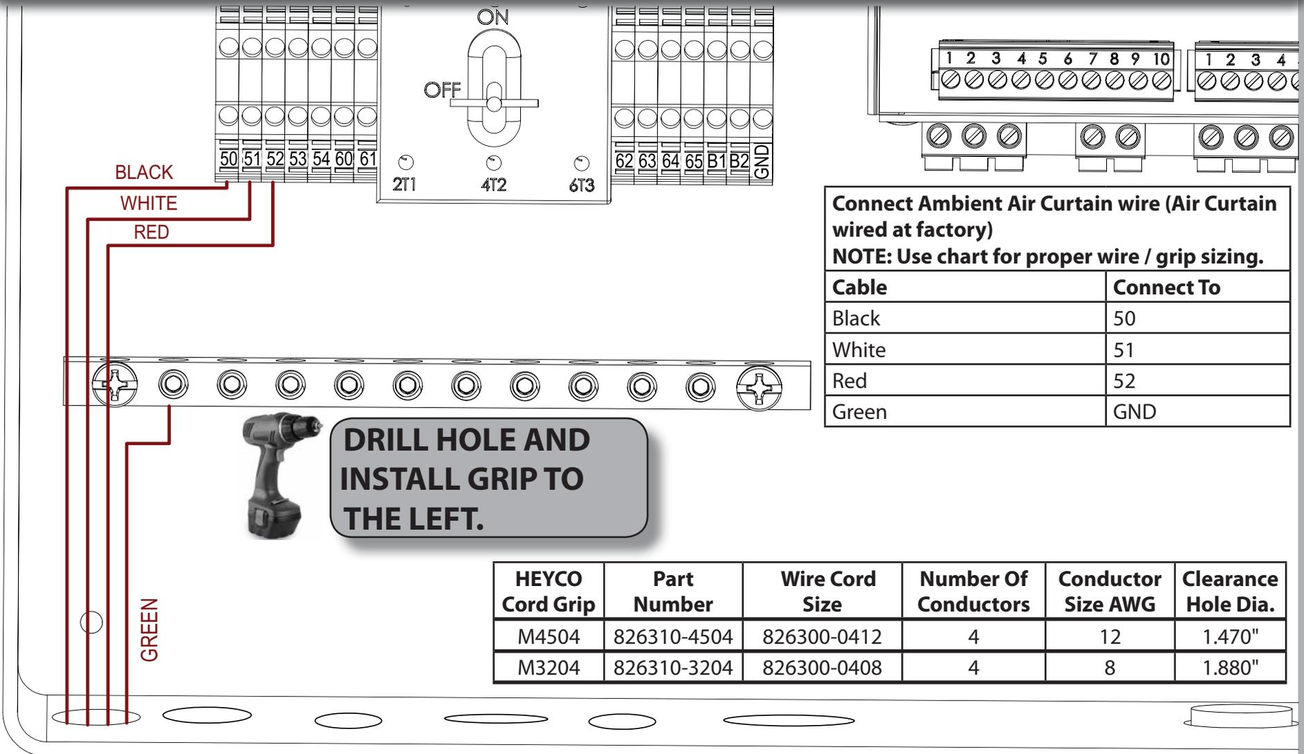
**Connect Ambient Air Curtain wire (Air Curtain wired at factory)**
