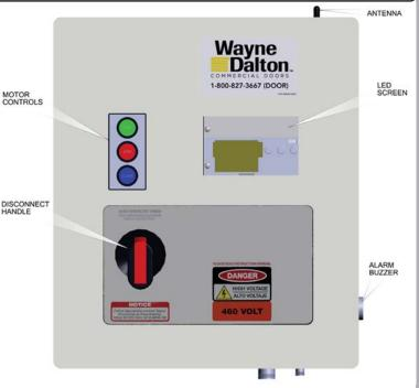
C. Once in the main screen, a 25 second countdown timer will show on the upper left hand corner. This countdown timer displays how long until the OPEN/STOP/CLOSE buttons will no longer give access to the MENU. Once inside the menu, use the **OPEN button to scroll up, STOP button to enter,** and **CLOSE to scroll down.** Pressing OPEN/STOP/CLOSE immediately exits the counter.
