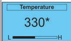
Temperature shows the internal temperature of the DGII Controller. This is a raw analog value and does not represent degrees centigrade or Fahrenheit. A display on the bottom graphically approximates either a Low or High temperature
