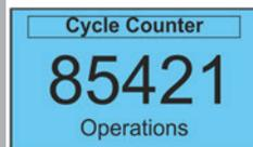
Cycle counter shows the number of operating cycles the door has completed (open/close = 1 cycle). Note: This is already shown by default at the top left corner in the main screen.
