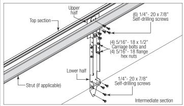
**FOR DOOR SECTIONS WITH ALL WINDOWS INSTALLATION:** Slide the top halve of the drawbar operator bracket assembly under the strut. Slide the bottom halve of the drawbar operator bracket assembly under the strut and over the center hinge, keeping the drawbar operator bracket assembly aligned with the center line. Attach the drawbar operator bracket assembly to the top section using 1/4" - 20 x 7/8" self drilling screws and strut clips.
