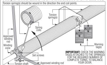
**FOR 6" AND DUPLEX SPRINGS:** Securely hold the winding rod while tightening the 4 set screws in the winding cone to 25 ft-lbs of torque (once set screws contact the torsion shaft, tighten an additional 1/2 turn).
