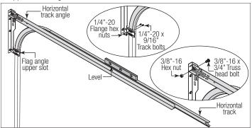
**IF YOU HAVE ANGLE MOUNT:** To install horizontal track, place the curved end over the top track roller of the top section. Align the bottom of the horizontal track with the top of the vertical track. Tighten the horizontal track to the angle mount with (2) 1/4" - 20 x 9/16" track bolts and (2) 1/4" - 20 flange hex nuts.
