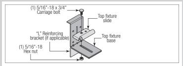
Starting on the left hand side of the top section, align the lip of the top fixture base on top of the corner of the top section and even with the edge of the section.
