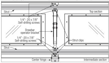
**NOTE:** Depending on your door width, it may be required that the rectangular drawbar operator bracket be mounted off center so the drawbar operator bracket mounts to the hinge points.
