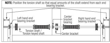
**IF YOUR DOOR HAS A COUPLER ASSEMBLY:** With assistance and starting on the left hand side of door, pick up the left hand torsion spring assembly and slide one end of the torsion keyed shaft through the end bearing bracket. Lay the other side of the torsion keyed shaft into the center bracket. Repeat the same process for the right hand torsion spring assembly. Position both torsion keyed shafts so that equal amounts of the shafts extend from each of the end bearing brackets.
