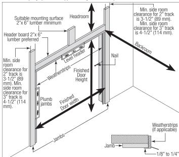
**HEADROOM REQUIREMENT:** Headroom is defined as the space needed above the top of the door for tracks, springs, etc. to allow the door to open properly. If the door is to be motor operated, 2-1/2" (64 mm) of additional headroom is required.
