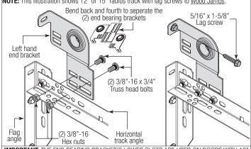
IMPORTANT: THE END BEARING BRACKET'S LOWER SLOTS ARE USED ON DOORS WITH 12 RADIUS TRACK: THE UPPER SLOTS ARE USED ON DOORS WITH 15" RADIUS TRACK.
