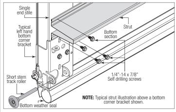
**NOTE:** If you have broken cable safety devices, only install the top (4) 1/4" - 14 x 7/8" self drilling screws to secure the bottom corner bracket to the bottom section. Reference Step
