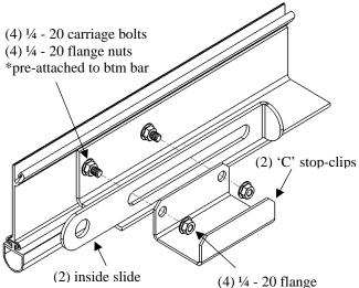
III: 'C' Stop-Clip w/ Inside Slide Bolt Attachment:
