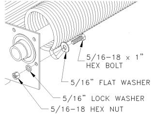
(Axle Pin installed in step #5 omitted from view for clarity)
