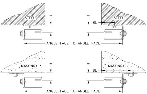
**packing slip**. Use this measurement to locate the left hand wall angle on the left hand jamb and clamp in place. Install bolts in the top and bottom holes in the wall angle. Verify that both wall angles are plumb and parallel, by double checking the angle to angle measurement at the top, middle, and bottom. Using a string and a level, ensure that the mounting angles are level to each other, shimming if necessary, to achieve horizontal level.
