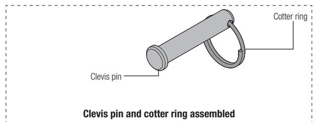
Clevis pin and cotter ring assembled
