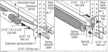
**NOTE:** As an option, eyebolt may be fastened to rear back hangs and extension spring bracket left unused. The extension spring bracket is useful in applications where rear headroom is small, resulting in short rear back hangs.
