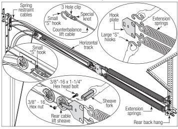
**IMPORTANT:** CLOSE "S" HOOKS AND EYE BOLTS WITH LOCKING PLIERS, TO PREVENT SPRINGS FROM COMING LOOSE.
