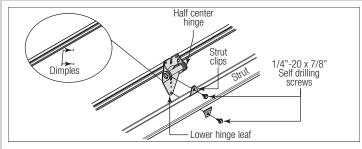
**IMPORTANT:** ONCE THE 1/4" - 20 SELF DRILLING SCREWS ARE SNUG AGAINST THE LOWER HINGE LEAFS, TIGHTEN AN ADDITIONAL 1/4 TO 1/2 TURN TO RECEIVE MAXIMUM DESIGN HOLDING POWER.
