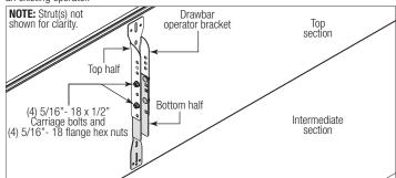
**FOR STANDARD INSTALLATION:** Slide the top halve of the drawbar operator bracket assembly under the strut, keeping the drawbar operator bracket assembly aligned with the center line. Remove the strut's screws, if necessary and attach to the top section (through strut if necessary) using (3) 1/4" - 20 x 7/8" self drilling screws.
