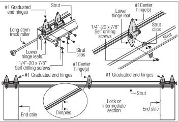
**NOTE:** If a strut is required to be installed on a section with windows in it, half center hinge(s) (if included) may need to be used instead of the typical center hinge(s).
