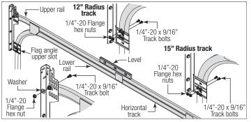
Next level the horizontal track assembly and bolt the top rail of the horizontal track to the encountered slot in the flag angle using (1) 1/4" -  $20 \times 9/16$ " track bolt, (1) 1/4" - 20 flange hex nut and (1) 5/16" washer. Repeat for other side.
