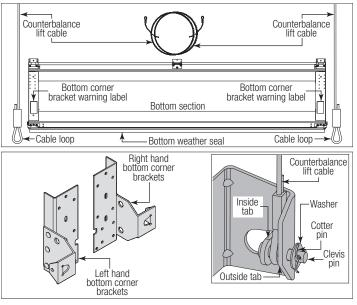
Position the left hand bottom corner bracket onto the bottom section. Attach the bottom corner bracket to the bottom section with (3) 1/4" - 20 x 11/16" RED HEAD self drilling screws and (2) 1/4" - 20 x 11/16" self drilling screws, as shown. Repeat same process for the right hand side.
