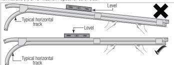
Next remove the nail that was temporarily holding the top section in place, installed in step, Top Section
