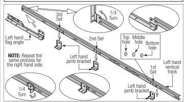
**FOR DOORS WITH FULLY ADJUSTABLE TRACK:** Hand tighten the left hand flag angle to the left hand vertical track using (2) 1/4" -  $20 \times 9/16$ " track bolts and (2) 1/4" - 20 flange hex nuts.
