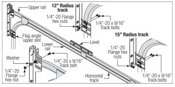
Next level the horizontal track assembly and bolt the top rail of the horizontal track to the encountered slot in the flag angle using (1) 1/4" - 20 x 9/16" track bolt, (1) 1/4" - 20 flange hex nut and (1) 5/16" washer. Repeat for other side.
