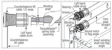
**FOR SINGLE SPRING APPLICATIONS:** Insert the idler bracket into the left hand cable drum. Lightly press the idler bracket into the cable drum until two distinct clicks are heard, or the bracket is inserted all the way.
