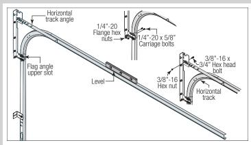
Next level the horizontal track assembly and bolt the horizontal track angle to the first encountered slot in the flag angle using (1) 3/8" -  $16 \times 3/4$ " hex head bolt and (1) 3/8" -  $16 \times 10$  hex nut. Repeat for other side. Remove nail that was temporally holding the top section in position.
