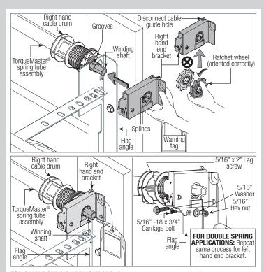
**FOR SINGLE SPRING APPLICATIONS:** Secure the idler bracket to the flag angle using (1) 5/16" - 18 x 3/4" carriage bolt, (1) 5/16" washer and (1) 5/16" - 18 hex nut. Then secure the idler bracket to the jamb using (1) 5/16" x 2" lag screw.
