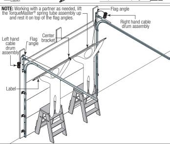
**NOTE:** Cable drum assemblies are marked right and left hand. Cable drums and TorqueMaster® spring tube assembly are cam shaped to fit together only one way.
