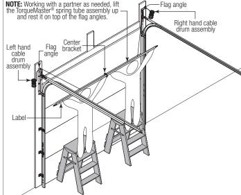
**NOTE:** Cable drum assemblies are marked right and left hand. Cable drums and TorqueMaster® spring tube assembly are cam shaped to fit together only one way.
