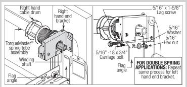
**FOR SINGLE SPRING APPLICATIONS:** Secure the idler bracket to the flag angle using (1) 5/16" - 18 x 3/4" carriage bolt, (1) 5/16" washer and (1) 5/16" - 18 hex nut. Then secure the idler bracket to the jamb using (1) 5/16" x 1-5/8" lag screw.
