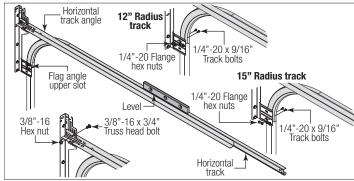
Next level the horizontal track assembly and bolt the horizontal track angle to the first encountered slot in the flag angle / angle mount using (1)  $3/8" - 16 \times 3/4"$  truss head bolt and (1) 3/8" - 16 hex nut. Repeat for other side. Remove nail that was temporally holding the too section in position.
