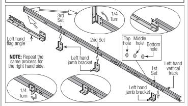
**FOR DOORS WITH FULLY ADJUSTABLE TRACK:** Hand tighten the left hand flag angle to the left hand vertical track using (2) 1/4" - 20 x 9/16" track bolts and (2) 1/4" - 20 flange hex nuts.
