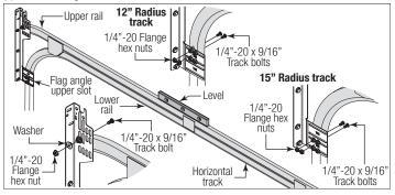
IF YOU HAVE ANGLE MOUNT VERTICAL TRACK ASSEMBLIES: To install horizontal track, place the top rail end over the top track roller of the top section. Align the bottom rail end of the horizontal track with the top of the vertical track. Tighten the bottom rail of the horizontal track to the angle mount with (2) 1/4" -  $20 \times 9/16$ " track bolts and (2) 1/4" -  $20 \inf(1/4)$ " - 20
