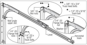
Next level the horizontal track assembly and bolt the top rail of the horizontal track to the encountered slot in the flag angle / angle mount using (1) 1/4" -  $20 \times 9/16$ " track bolt, (1) 1/4" - 20 flange hex nut and (1) 5/16" washer.
