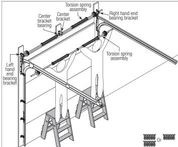
With assistance, pick up the torsion spring assembly and slide one end of the torsion shaft through one end bearing bracket. Lay the middle of the torsion shaft into the center bracket. Slide the other end of the torsion shaft into the other end bearing bracket. Position the torsion shaft so that equal amounts of the shaft extend from each end bearing bracket.
