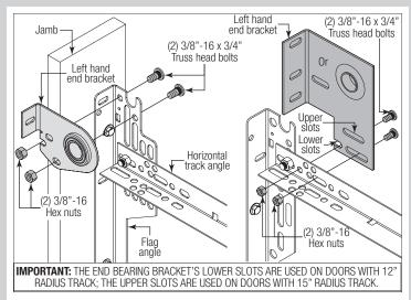
Secure the top of the end bearing bracket to the jamb using 5/16" x 1-5/8" lag screw(s). Repeat the same process for right hand side.
