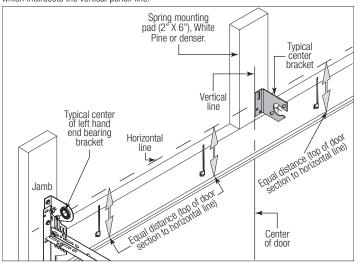
IF YOUR DOOR DID NOT COME WITH A CENTER COUPLER ASSEMBLY OR TORSION SPRINGS LESS THAN 3-3/4" ID: Mark a vertical pencil line on the mounting surface above the door, at the center. Align the edge of the center bracket with the vertical pencil line and
