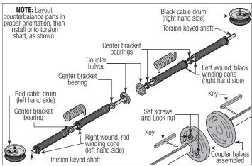
With assistance and starting on the left hand side of door, pick up the left hand torsion spring assembly and slide one end of the torsion keyed shaft through the end bearing bracket. Lay the other side of the torsion keyed shaft into the center bracket. Repeat the same process for the right hand torsion spring assembly.
