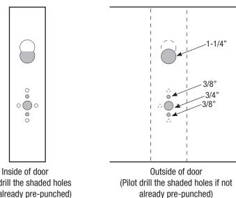
Use noted holes to pilot drill thru the exterior if prepunched holes are not in section.
