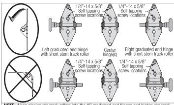
**NOTE:** When placing the track rollers into the #2 graduated end hinges and higher, the track roller goes into the hinge tube furthest away from the section.
