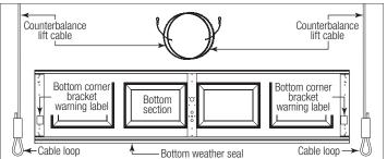
Locate the left hand bottom corner bracket. Slide the left hand cable loop of the counterbalance lift cable onto milford pin. Position the left hand bottom corner bracket onto the bottom section. Attach the bottom corner bracket to the bottom section with (3) 1/4" - 20 x 11/16" RED HEAD self drilling screws. Repeat same process for the right hand side.
