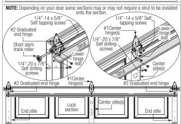
Insert a short stem track roller into the hinge tube of the graduated end hinges. Repeat graduated hinge attachment using the appropriate graduated end hinges for all remaining sections except the top section.
