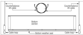
**NOTE:** Refer to Strutting Schedule (shown on the Windload Specification Sheet), to determine if a strut needs to be installed on top of the bottom corner brackets at the bottom portion of the bottom section.
