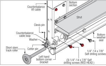
**IMPORTANT:** THE 1/4" - 14 X 7/8" RED HEAD SELF DRILLING SCREWS MUST BE MUST BE INSTALLED THROUGH THE HOLES OF THE BOTTOM CORNER BRACKETS, AS SHOWN.
