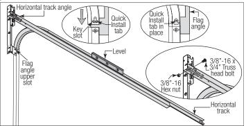
**FOR OTHER FLAG ANGLES:** To install horizontal track, place the curved end over the top track roller of the top section. Align the bottom of the horizontal track with the top of the vertical track. Tighten the horizontal track to the flag angle with (2)  $1/4" - 20 \times 9/16"$  track bolts and (2) 1/4" - 20 flange hex nuts.
