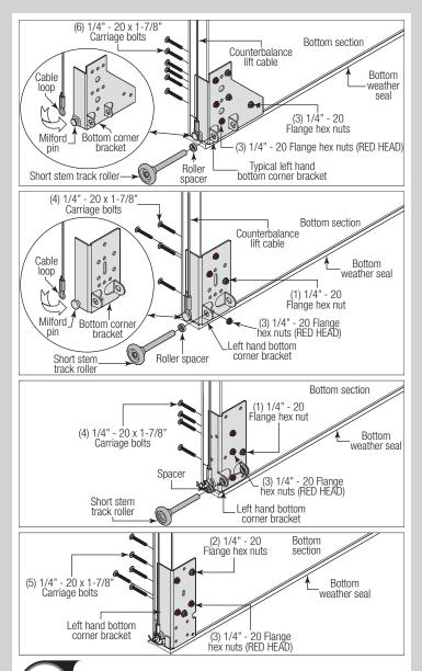
Attaching Track Roller Carrier's
