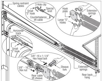
**IMPORTANT:** CLOSE "S" HOOKS AND EYE BOLTS WITH LOCKING PLIERS, TO PREVENT SPRINGS FROM COMING LOOSE.
