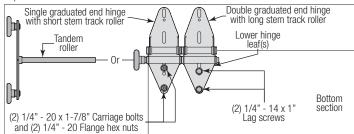
**FOR GRADUATED END HINGES WITH A LONG STRUT:** Attach the upper leg of the strut, (1) strut clip to the upper slot of the graduated end hinge to the bottom section using (1)  $1/4" - 20 \times 1-7/8"$  carriage bolt and (1) 1/4" - 20 flange hex nut. Secure the lower leg of the strut, (1) strut clip to the lower hole of the graduated end hinge to the bottom section using (1)  $1/4" - 20 \times 1-7/8"$  carriage bolt and (1) 1/4" - 20 flange hex nut. Repeat for other side.
