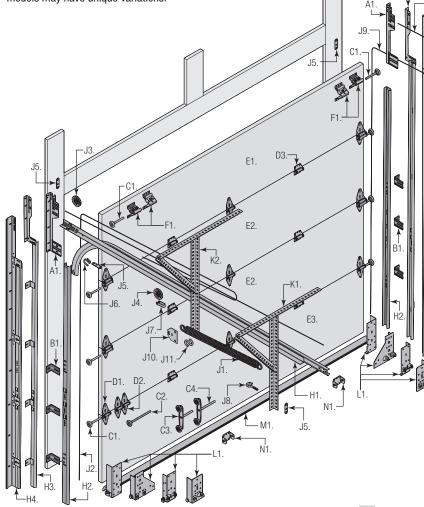
**NOTE:** For Item (K2), The Rear Center Back Hang Assemblies are to used for all doors over 11'0" door height and over 14'0" door width. One Rear Center Back Hang Assembly, per side.
