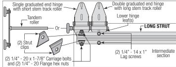
**FOR CENTER HINGES WITHOUT A LONG STRUT:** Attach the upper slot of the center hinge to the Intermediate section using (1)  $1/4" - 20 \times 1-7/8"$  carriage bolt and (1) 1/4" - 20 flange hex nut. Secure the lower hole of the center hinge to the Intermediate section using (1)  $1/4" - 20 \times 1-7/8"$  carriage bolt and (1) 1/4" - 20 flange hex nut. Repeat for other center hinge(s).
