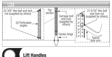
NOTE: Lift handles must be lined up vertically.
