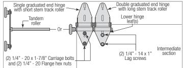
**FOR GRADUATED END HINGES WITH A LONG STRUT:** Attach the upper leg of the strut, (1) strut clip to the upper slot of the graduated end hinge to the Intermediate section using (1)  $1/4" - 20 \times 1-7/8"$  carriage bolt and (1) 1/4" - 20 flange hex nut. Secure the lower leg of the strut, (1) strut clip to the lower hole of the graduated end hinge to the Intermediate section using (1)  $1/4" - 20 \times 1-7/8"$  carriage bolt and (1) 1/4" - 20 flange hex nut. Repeat for other side.
