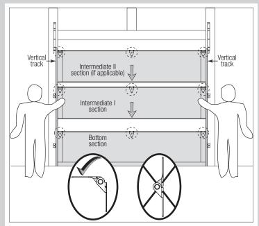
**FOR CENTER HINGE(S):** Starting with a center hinge, flip the upper hinge leaf up. If needed use it as a template, mark and pre-drill (2) 9/32" diameter holes through the section. Attach the upper hinge leaf to the section using (2)  $1/4" - 20 \times 1-7/8"$  carriage bolts and (2) 1/4" - 20 flange hex nuts. Repeat same process for the other Center Hinges.
