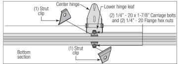
**NOTE:** If you don't have half center hinges, then skip this part of the step. Refer to Package Contents / Breakdown Of Parts, to determine if you have half center hinges. Using a tape measure, position the half center hinges equally spaced in between the center
