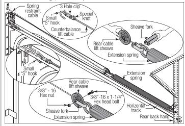
**NOTE:** Some larger doors feature 2 pairs of extension springs. A spring restraint cable must be installed through each spring.
