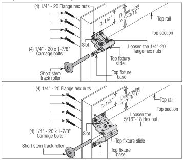
FOR TOP SECTIONS WITH A <u>3-1/8" TOP RAIL:</u> Measure down from the top of the top section 1-1/8" and make a small mark. Align the top of the top fixture assembly with the mark previously made and even with the edge of the section.
