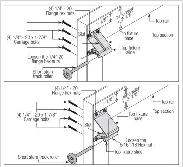
**NOTE:** Ensure the top fixture slide is able to slide along the top fixture base. If needed, loosen the 1/4" - 20 flange hex nuts.
