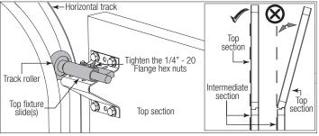
If needed. lock each of the top fixture slides into place using (1) 1/4" - 20 x 9/16" track bolt and (1) 1/4" - 20 flange hex nut through any two aligning holes.
