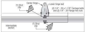
**NOTE:** If you don't have half center hinges, then skip this part of the step. Refer to Package Contents / Breakdown Of Parts, to determine if you have half center hinges.
