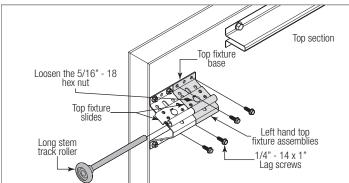
Insert the appropriate short / long stem track roller into the top fixture slide(s).
