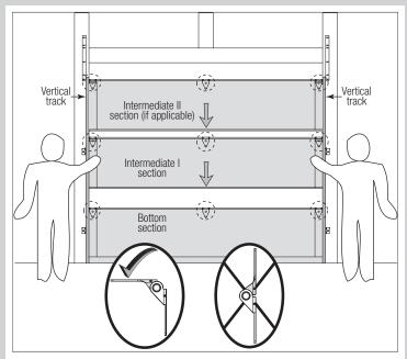
**FOR CENTER HINGE(S):** Starting with a center hinge, flip the upper hinge leaf up. If needed use it as a template, mark and pre-drill (2) 9/32" diameter holes through the section. Attach the upper hinge leaf to the section using (2) 1/4" - 20 x 1-7/8" carriage bolts and (2) 1/4" - 20 flange hex nuts. Repeat same process for the other Center Hinges.
