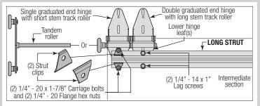
**FOR CENTER HINGES WITHOUT A LONG STRUT:** Attach the upper slot of the center hinge to the Intermediate section using (1) 1/4" -  $20 \times 1$ -7/8" carriage bolt and (1) 1/4" - 20 flange hex nut. Secure the lower hole of the center hinge to the Intermediate section using (1) 1/4" -  $20 \times 1$ -7/8" carriage bolt and (1) 1/4" - 20 flange hex nut. Repeat for other center hinge(s).
