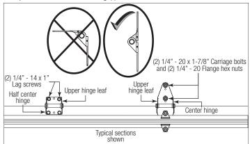
**FOR GRADUATED END HINGES:** Starting with the outer graduated end hinges, flip the upper hinge leaf up. If needed use it as a template, mark and pre-drill (2) 9/32" diameter holes through the section. Attach the upper hinge leaf to the section using (2) 1/4" - 20 x 1-7/8" carriage bolts and (2) 1/4" - 20 flange hex nuts. Repeat same process for the other side.
