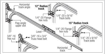
IF YOU HAVE ANGLE MOUNT: To install horizontal track, place the curved end over the top track roller of the top section. Align the bottom of the horizontal track with the top of the vertical track. Tighten the horizontal track to the angle mount with (2) 1/4" -  $20 \times 9/16$ " track bolts and (2) 1/4" - 20 flange hex nuts.
