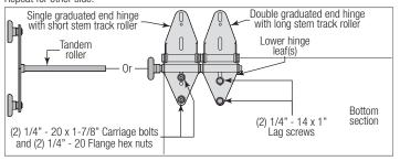
**FOR CENTER HINGES:** Attach the upper slot of the graduated end hinge to the bottom section using (1) 1/4" -  $20 \times 1$ -7/8" carriage bolt and (1) 1/4" - 20 flange hex nut. Next attach the bottom hole of the graduated end hinge to the bottom section using (1) 1/4" -  $20 \times 1$ -7/8" carriage bolt and (1) 1/4" - 20 flange hex nut.
