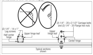
**FOR GRADUATED END HINGES:** Starting with the outer graduated end hinges, flip the upper hinge leaf up. If needed use it as a template, mark and pre-drill (2) 9/32" diameter holes through the section. Attach the upper hinge leaf to the section using (2) 1/4" -  $20 \times 2-1/2$ " carriage bolts and (2) 1/4" -  $20 \times 10^{-1}$  flange hex nuts. Repeat same process for the other side.
