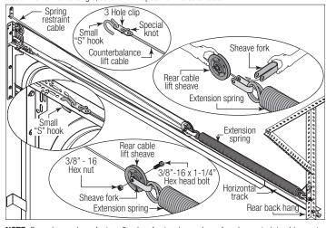
$\mbox{\bf NOTE:}$  Some larger doors feature 2 pairs of extension springs. A spring restraint cable must be installed through each spring.
