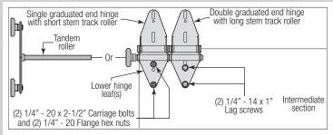
**FOR GRADUATED END HINGES WITH A LONG STRUT:** Attach the upper leg of the strut, (1) strut clip to the upper slot of the graduated end hinge to the Intermediate section using (1) 1/4" -  $20 \times 2$ -1/2" carriage bolt and (1) 1/4" - 20 flange hex nut. Secure the lower leg of the strut, (1) strut clip to the lower hole of the graduated end hinge to the Intermediate section using (1) 1/4" -  $20 \times 2$ -1/2" carriage bolt and (1) 1/4" - 20 flange hex nut. Repeat for other side.
