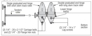
**FOR CENTER HINGES:** Attach the upper slot of the graduated end hinge to the bottom section using (1) 1/4" -  $20 \times 2$ -1/2" carriage bolt and (1) 1/4" - 20 flange hex nut. Next attach the bottom hole of the graduated end hinge to the bottom section using (1) 1/4" -  $20 \times 2$ -1/2" carriage bolt and (1) 1/4" - 20 flange hex nut.
