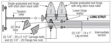
**FOR CENTER HINGES WITHOUT A LONG STRUT:** Attach the upper slot of the center hinge to the Intermediate section using (1) 1/4" - 20 x 2-1/2" carriage bolt and (1) 1/4" - 20 flange hex nut. Secure the lower hole of the center hinge to the Intermediate section using (1) 1/4" - 20 x 2-1/2" carriage bolt and (1) 1/4" - 20 flange hex nut. Repeat for other center hinge(s).
