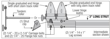
**FOR CENTER HINGES:** Align the slots of the lower hinge leaf with the pre-drilled holes at each center stile, located at the top rail of the Intermediate section. Using the center hinge as a template, drill pilot holes, 1" deep into the Intermediate section with a 1/8" drill bit (if needed).
