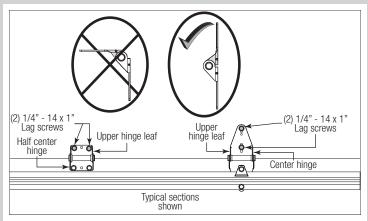
**FOR GRADUATED END HINGES:** Starting with the outer graduated end hinges, flip the upper hinge leaf up and use it as a template. Mark and pre-drill (2) 9/32" diameter holes through the section. Attach the upper hinge leaf to the section using (2) 1/4" - 20 x 2-1/4" carriage bolts and (2) 1/4" - 20 flange hex nuts. Repeat same process for the other side.
