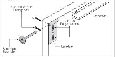
**IF YOU HAVE FOUR TOP FIXTURE ASSEMBLIES:** Position the second top fixture assembly next to the first installed top fixture assembly. Using the top fixture base as a template, drill pilot holes, 1" deep into the top section with a 1/8" drill bit (if needed).
