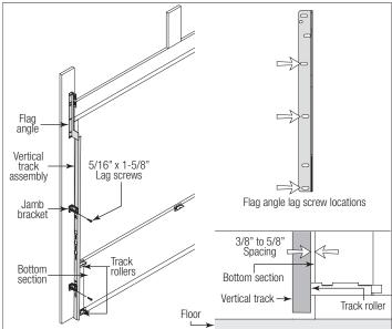
**FOR RIVETED VERTICAL TRACK ASSEMBLY:** Loosely fasten jamb brackets and flag angle to the jamb using 5/16" x 1-5/8" lag screws. Tighten lag screws, securing the bottom jamb bracket to jamb, maintain 3/8" to 5/8" spacing as shown between the bottom section and vertical track. Hang counterbalance lift cable over flag angle. Repeat same process for other side.
