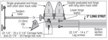
**FOR CENTER HINGES:** Align the slots of the lower hinge leaf with the pre-drilled holes at each center stile, located at the top rail of the bottom section. Using the center hinge as a template, drill pilot holes, 1" deep into the bottom section with a 1/8" drill bit (if needed).
