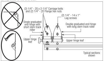
**IMPORTANT:** PUSH & HOLD THE HINGE LEAFS SECURELY AGAINST THE SECTIONS WHILE SECURING WITH APPROPRIATE FASTENERS. THERE SHOULD BE NO GAP BETWEEN THE HINGE LEAFS AND THE SECTIONS.
