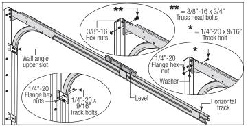
Next level the horizontal track assembly and bolt the top rail of the horizontal track to the encountered slot in the flag angle / angle mount using (1) 1/4" - 20 x 9/16" track bolt, (1) 1/4" - 20 flange hex nut and (1) 5/16" washer.
