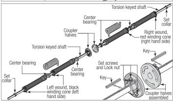
With assistance and starting on the left hand side of door, pick up the left hand torsion spring assembly and slide one end of the torsion keyed shaft through the end bearing bracket. Lay the other side of the torsion keyed shaft into the center bracket. Repeat the same process for the right hand torsion spring assembly. Position both torsion keyed shafts so that equal amounts of the shafts extend from each end bearing brackets.
