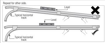
Next remove the nail that was temporarily holding the top section in place, installed in step, Top Section.
