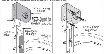
Position the left hand end bearing bracket up against the jamb and on the horizontal track, as shown. Fasten the left hand end bearing bracket to the horizontal track with (1) 3/8" - 16 x 3/4" truss head bolt and (1) 3/8" - 16 nut. Secure the left hand end bearing bracket to the jamb using (3) 5/16" x 1-5/8" lag screws. Repeat same process for the other side.
