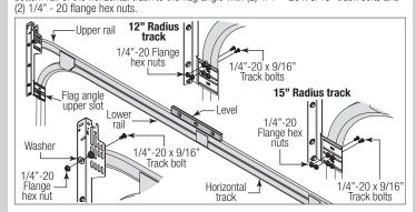
**IF YOU HAVE ANGLE MOUNT VERTICAL TRACK ASSEMBLIES:** To install horizontal track, place the top rail end over the top track roller of the top section. Align the bottom rail end of the horizontal track with the top of the vertical track. Tighten the bottom rail of the horizontal track to the angle mount with (2) 1/4" - 20 x 9/16" track bolts and (2) 1/4" - 20 flange hex nuts.
