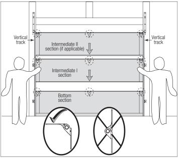
**FOR CENTER HINGE(S) AND OR HALF CENTER HINGE(S):** Flip a upper hinge leaf up and use it as a template. Mark and pre-drill (2) 1/8" pilot holes, 1" deep into the section with a 1/8" drill bit
