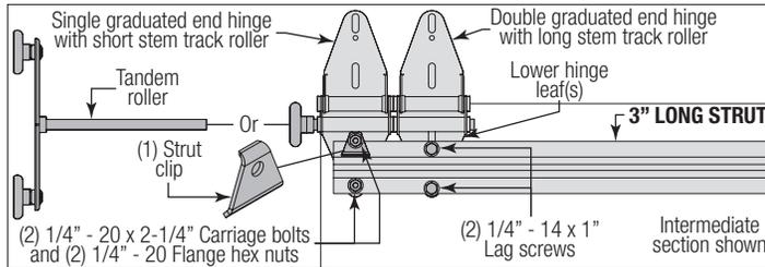
**FOR CENTER HINGES:** Align the slots of the lower hinge leaf with the pre-drilled holes at each center stile, located at the top rail of the Intermediate section. Using the center hinge as a template, drill pilot holes, 1" deep into the Intermediate section with a 1/8" drill bit (if needed).
