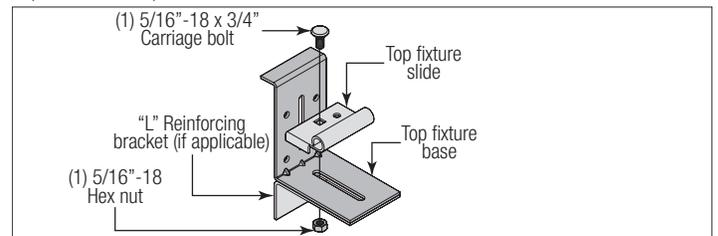
Starting on the left hand side, align the lip of the top fixture base onto the top corner of the top section and even with the side edge of the top section. Using the top fixture base as a template, mark and pre-drill (3) 9/32" diameter holes through the top section.
