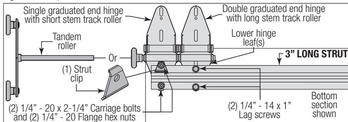
**FOR CENTER HINGES:** Align the slots of the lower hinge leaf with the pre-drilled holes at each center stile, located at the top rail of the bottom section. Using the center hinge as a template, drill pilot holes, 1" deep into the bottom section with a 1/8" drill bit (if needed).
