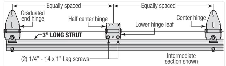
If you have single graduated end hinges, insert a short stem track roller / short stem tandem track roller (if included) into the hinge tube on each side.
