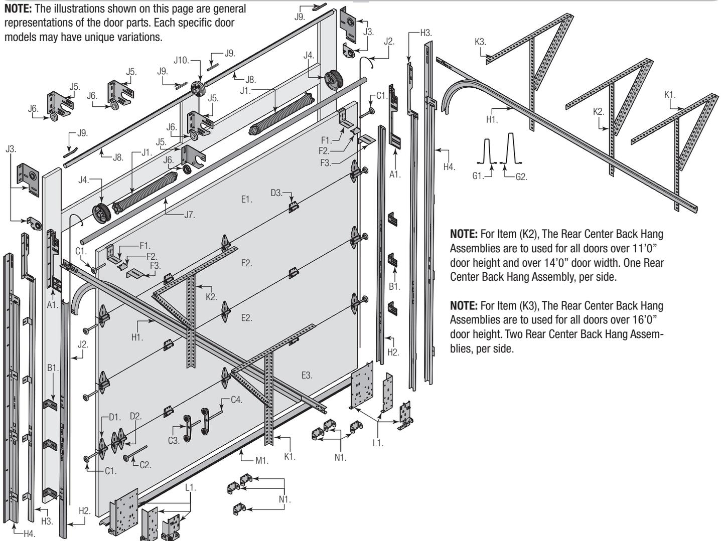
**NOTE:** For Item (K2), The Rear Center Back Hang Assemblies are to be used for all doors over 11'0" door height and over 14'0" door width. One Rear Center Back Hang Assembly, per side.
