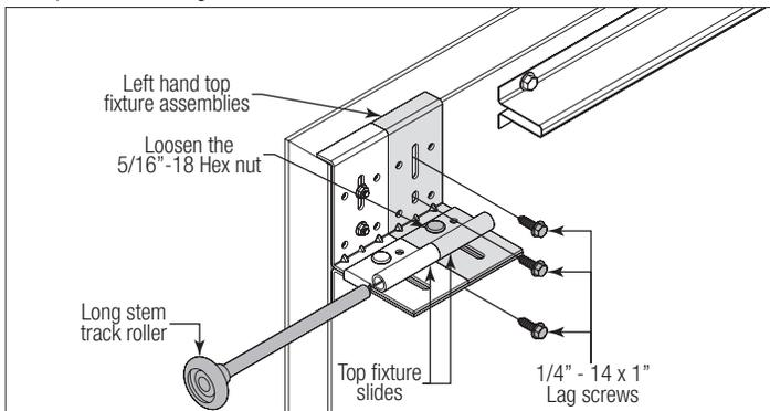
ASSEMBLY SHOULD BE INSTALLED SUCH THAT WHEN THE FLOOR IS CONSTRUCTED, NO DOOR OR TRACK PARTS ARE TRAPPED IN THE FLOOR CONSTRUCTION.
