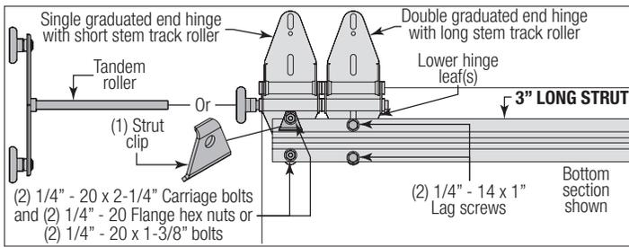
**FOR CENTER HINGES:** Align the slots of the lower hinge leaf with the pre-drilled holes at each center stile, located at the top rail of the bottom section. Using the center hinge as a template, drill pilot holes, 1" deep into the bottom section with a 1/8" drill bit (if needed).
