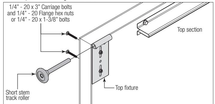
**IF YOU HAVE FOUR TOP FIXTURE ASSEMBLIES:** Position the second top fixture assembly next to the first installed top fixture assembly. Using the top fixture base as a template, drill pilot holes, 1" deep into the top section with a 1/8" drill bit (if needed).
