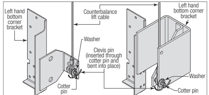
Locate the left hand bottom corner bracket. Align the bottom corner bracket horizontally with the bottom edge of the bottom section and align the bottom corner bracket vertically with the left bottom edge of the bottom section.
