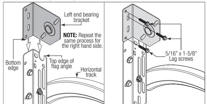
Position the left hand end bearing bracket up against the jamb and on the horizontal track, as shown. Fasten the left hand end bearing bracket to the horizontal track with (1) 3/8" - 16 x 3/4" truss head bolt and (1) 3/8" - 16 nut. Secure the left hand end bearing bracket to the jamb using (3) 5/16" x 1-5/8" lag screws. Repeat same process for the other side.
