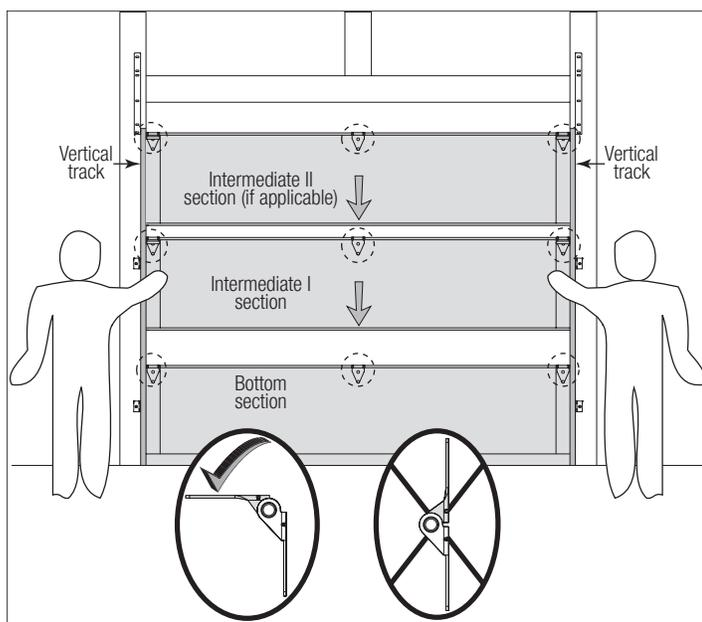
**NOTE:** Refer to the Schedules below, to determine if your doors requires strutting, prior to attaching sections.
