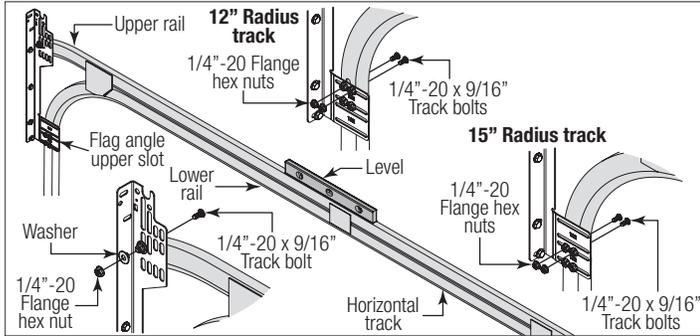
**IF YOU HAVE ANGLE MOUNT VERTICAL TRACK ASSEMBLIES:** To install horizontal track, place the top rail end over the top track roller of the top section. Align the bottom rail end of the horizontal track with the top of the vertical track. Tighten the bottom rail of the horizontal track to the angle mount with (2) 1/4" - 20 x 9/16" track bolts and (2) 1/4" - 20 flange hex nuts.
