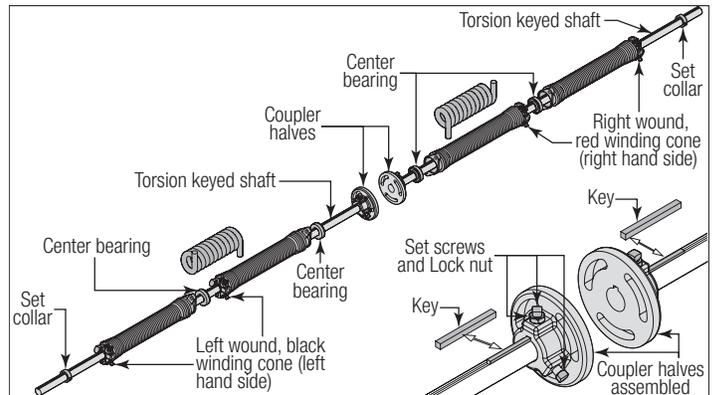
With assistance and starting on the left hand side of door, pick up the left hand torsion spring assembly and slide one end of the torsion keyed shaft through the end bearing bracket. Lay the other side of the torsion keyed shaft into the center bracket. Repeat the same process for the right hand torsion spring assembly. Position both torsion keyed shafts so that equal amounts of the shafts extend from each end bearing brackets.
