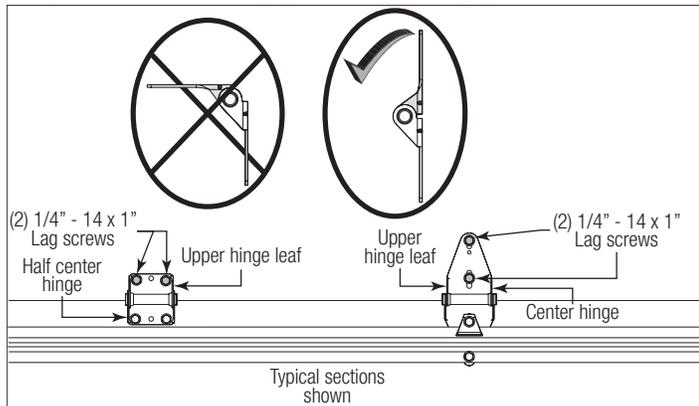
**FOR GRADUATED END HINGES:** Starting with the outer graduated end hinges, flip the upper hinge leaf up. If needed use it as a template, mark and pre-drill (2) 9/32" diameter holes through the section. Attach the upper hinge leaf to the section using (2) 1/4" - 20 x 3" carriage bolts and (2) 1/4" - 20 flange hex nuts or (2) 1/4" - 20 x 1-3/8" bolts. Repeat same process for the other side.
