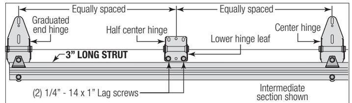
If you have single graduated end hinges, insert a short stem track roller / short stem tandem track roller (if included) into the hinge tube on each side.
