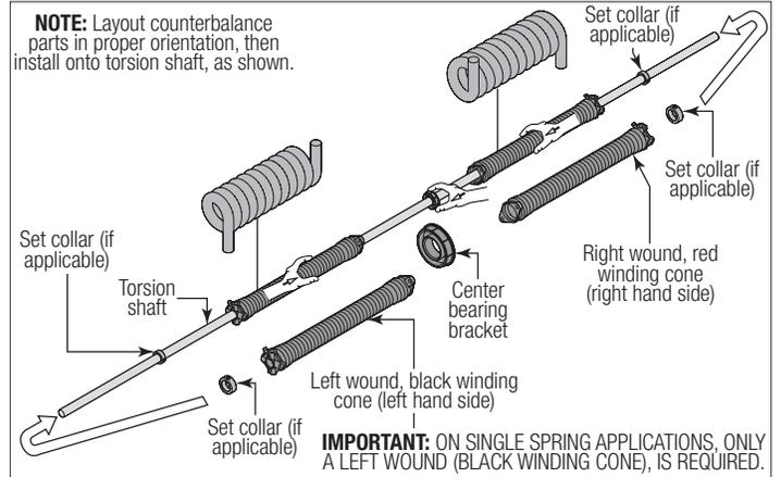
With assistance, pick up the torsion spring assembly and slide one end of the torsion shaft / torsion keyed shaft through one end bearing bracket. Lay the middle of the torsion shaft / torsion keyed shaft into the center bracket. Slide the other end of the torsion shaft / torsion keyed shaft into the other end bearing bracket. Position the torsion shaft / torsion keyed shaft so that equal amounts of the shaft extend from each end bearing bracket.
