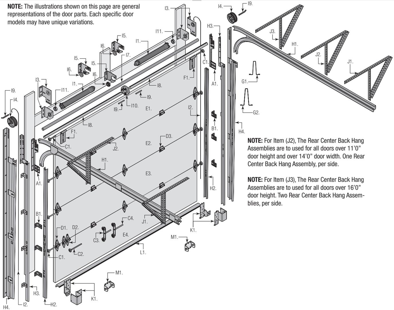
**NOTE:** For Item (J2), The Rear Center Back Hang Assemblies are to be used for all doors over 11'0" door height and over 14'0" door width. One Rear Center Back Hang Assembly, per side.
