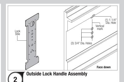
**8000 / 8100 / 8200 DOORS:** Align the outside handle assembly with the handle pointing towards the floor and insert the assembly through the previously drilled 3/4" diameter holes in the section. Secure the outside lock handle to the section with (2) #10 phillips head screws.
