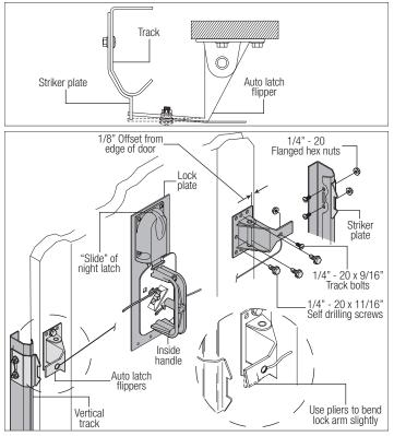
Operate the lock several times to make sure the auto latch flippers clear the striker plates when the handle is turned and the flippers engage the striker plates when the handle is released. Adjust the cables if necessary. Trim off the excess cable with wire cutters after the lock is operating satisfactorily.
