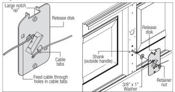
Place the lock plate over the 1-1/4" diameter center stile hole and fasten with (2) #12 pan head screws into the rim cylinder. In addition, align the night latch slide with the notch in the top of the release disk. Fasten the night latch to the center stile with (4) #8 x 1/2" pan head screws.
