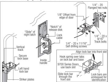
Operate the lock several times to make sure the lock bars clear the striker plates when the handle is turned and the lock bars engage the striker plates when the handle is released. Adjust the cables if necessary. Trim off the excess cable with wire cutters after the lock is operating satisfactorily.
