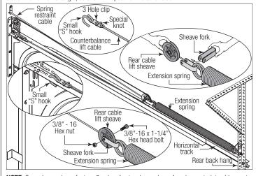
**NOTE:** Some larger doors feature 2 pairs of extension springs. A spring restraint cable must be installed through each spring.
