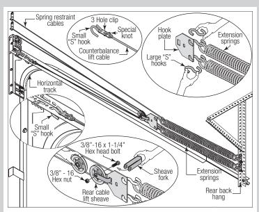
**IMPORTANT:** CLOSE "S" HOOKS AND EYE BOLTS WITH LOCKING PLIERS, TO PREVENT SPRINGS FROM COMING LOOSE.
