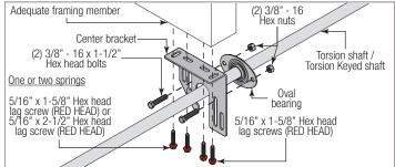
17 Attaching Torsion Spring
