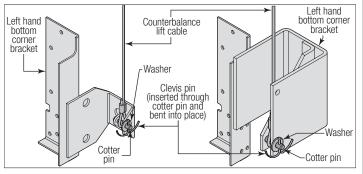
Locate the left hand bottom corner bracket. Align the bottom corner bracket horizontally with the bottom edge of the bottom section and align the bottom corner bracket vertically with the left bottom edge of the bottom section.
