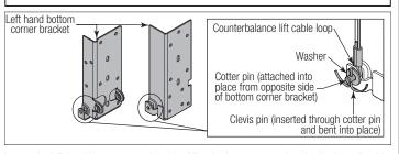
Locate the left hand bottom corner bracket. Align the bottom corner bracket horizontally with the bottom edge of the bottom section and align the bottom corner bracket vertically with the left bottom edge of the bottom section.
