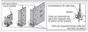
Locate the left hand bottom corner bracket. Align the bottom corner bracket horizontally with the bottom edge of the bottom section and align the bottom corner bracket vertically with the left bottom edge of the bottom section.
