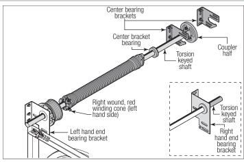
**NOTE:** Position both torsion keyed shafts so that equal amounts of the shafts extend from each end bearing brackets.
