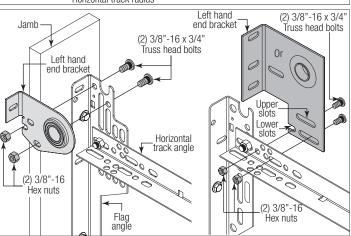
IMPORTANT: THE END BEARING BRACKET'S LOWER SLOTS ARE USED ON DOORS WITH 12' RADIUS TRACK; THE UPPER SLOTS ARE USED ON DOORS WITH 15" RADIUS TRACK.
