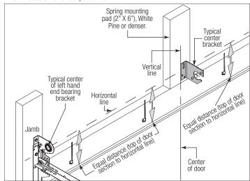
IF YOUR DOOR DID NOT COME WITH A CENTER COUPLER ASSEMBLY OR TORSION SPRINGS LESS THAN 3-3/4" ID: Mark a vertical pencil line on the mounting surface above the door, at the center. Align the edge of the center bracket with the vertical pencil line and the center of the center bracket with the horizontal pencil line; this is to ensure the torsion shaft is level between the center and end bearing brackets.
