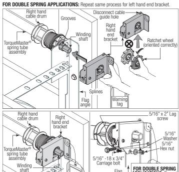
FOR SINGLE SPRING APPLICATIONS: Secure the idler bracket to the flag angle using (1) 5/16" - 18 x 3/4" carriage bolt, (1) 5/16" washer and (1) 5/16" - 18 hex nut. Then secure the idler bracket to the jamb using (1) 5/16" x 2" lag screw.
