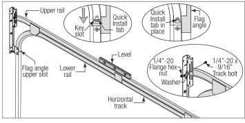
IF YOU HAVE FULLY ADJUSTABLE FLAG ANGLES OR RIVETED TRACK ASSEMBLIES: To install horizontal track, place the top rail end over the top track roller of the top section. Align the bottom rail end of the horizontal track with the top of the vertical track. Tighten the bottom rail of the horizontal track to the flag angle with (2) 1/4" - 20 x 9/16" track bolts and (2) 1/4" - 20 flange hex nuts.
