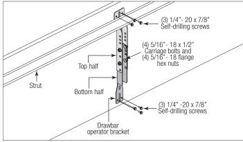
Locate the center of the top section. Position the drawbar operator bracket under the strut (if applicable) or align the drawbar operator bracket top edge with the top edge of the top section, as shown. Attach the drawbar operator bracket using (3) 1/4" - 20 x 7/8" self-drilling screws (as shown).
