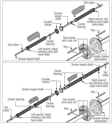
With assistance and starting on the left hand side of door, pick up the left hand torsion spring assembly and slide one end of the torsion keyed shaft through the end bearing bracket. Lay the other side of the torsion keyed shaft into the center bracket. Repeat the same process for the right hand torsion spring assembly. Position both torsion keyed shafts so that equal amounts of the shafts extend from each end bearing brackets.
