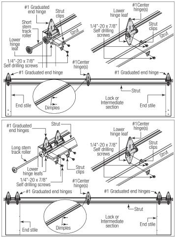
**NOTE:** If a strut is required to be installed on a section with windows in it, half center hinge(s) (if included) may need to be used instead of the typical center hinge(s).
