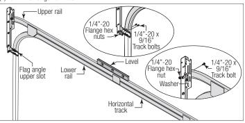
IF YOU HAVE ANGLE MOUNT VERTICAL TRACK ASSEMBLIES: To install horizontal track, place the top rail end over the top track roller of the top section. Align the bottom rail end of the horizontal track with the top of the vertical track. Tighten the bottom rail of the horizontal track to the angle mount with (2) 1/4" - 20 x 9/16" track bolts and (2) 1/4" - 20 flange hex nuts.
