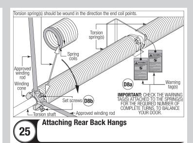
**IMPORTANT:** HOLD THE DOOR DOWN TO PREVENT IT FROM RISING UNEXPECTEDLY IN THE EVENT THE SPRING(S) WERE OVER-WOUND AND CAUTIOUSLY REMOVE LOCKING PLIERS FROM VERTICAL TRACKS.
