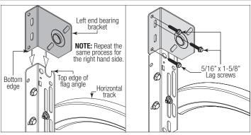
Position the left hand end bearing bracket up against the jamb and on the horizontal track, as shown. Fasten the left hand end bearing bracket to the horizontal track with (1)  $3/8" - 16 \times 3/4"$  truss head bolt and (1) 3/8" - 16 nut. Secure the left hand end bearing bracket to the jamb using (3)  $5/16" \times 1-5/8"$  lag screws. Repeat same process for the other side.
