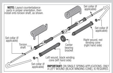
With assistance, pick up the torsion spring assembly and slide one end of the torsion shaft / torsion keyed shaft through one end bearing bracket. Lay the middle of the torsion shaft / torsion keyed shaft into the center bracket. Slide the other end of the torsion shaft / torsion keyed shaft into the other end bearing bracket. Position the torsion shaft / torsion keyed shaft so that equal amounts of the shaft extend from each end bearing bracket.
