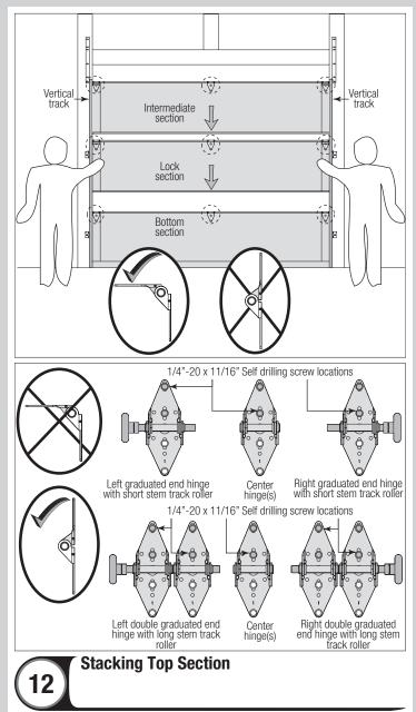
Place the top section in the opening. Install a nail to prevent the top section from falling backwards. Now, flip up the hinge leaves, hold tight against section, and fasten center hinges first and end hinges last (refer to step, Stacking Sections). Vertical track alignment is critical. Position flag angle or wall angle between 1-11/16" (43 mm) to 1-3/4" (44 mm) from the edge of the door; tighten the bottom lag screw. Flag angles must be parallel to the door sections. Repeat for other side.
