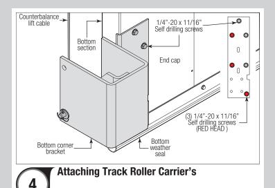
**NOTE:** If you don't have track roller carriers, then skip this step. Refer to Package Contents / Parts Breakdown of Parts, to determine if a track roller carrier was supplied with your door.
