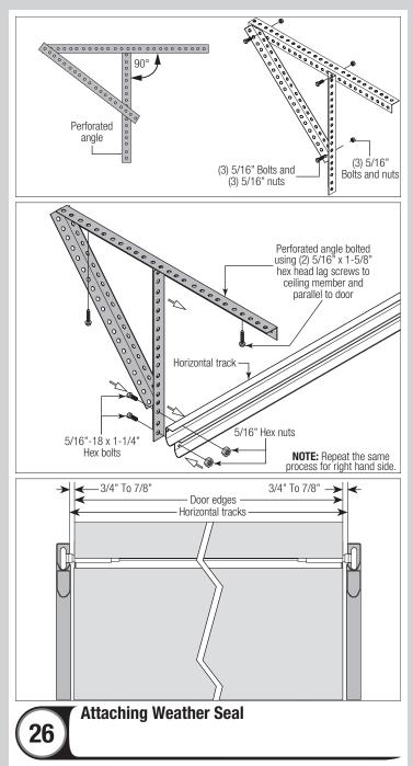
Permanently attach the weatherstrips on both door jambs and header. The weatherstrips were temporarily attached in Preparing the Opening, in the pre-installation section of this manual.
