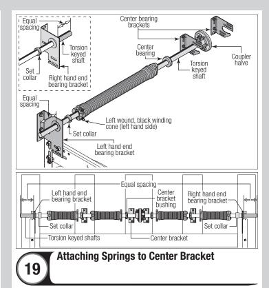
**IMPORTANT:** THE SPRING WARNING TAG(S) SUPPLIED MUST BE SECURELY ATTACHED TO THE STATIONARY SPRING CONE(S) IN PLAIN VIEW. SHOULD A REPLACEMENT SPRING WARNING TAG BE REQUIRED, CONTACT WAYNE DALTON FOR FREE REPLACEMENTS.
