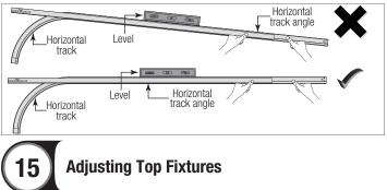
With horizontal tracks installed, you can now adjust the top fixtures. Vertically align the top section of the door with the lower sections. Once aligned, position the top fixture slide, out against the horizontal track. Maintaining the slide's position, tighten the (2) 1/4" - 20 flange hex nuts to secure the top fixture slide to the top fixture base. Repeat for other side.
