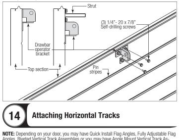
Angles, Riveted Vertical Track Assemblies or you may have Angle Mount Vertical Track Assemblies. Refer to Package Contents / Breakdown of Parts, to determine which Flag Angles / Vertical Track Assemblies you have.
